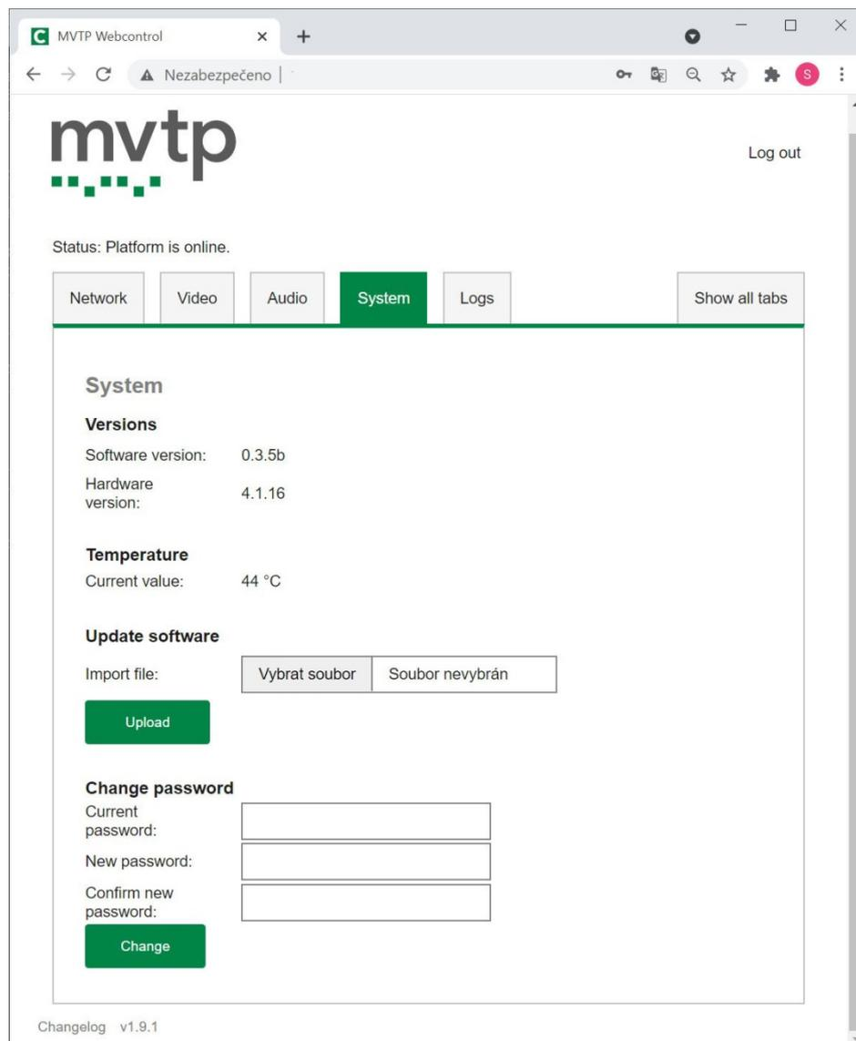
Fig. 5: System tab of the built-in web interface
