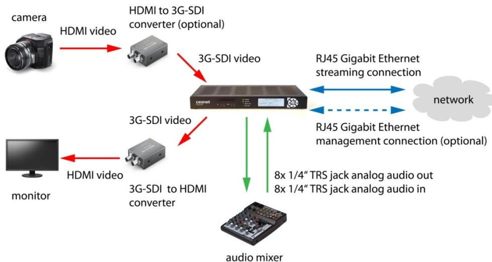
Fig. 1: Recommended connections of the MVTP-Audio device
