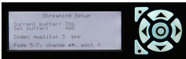
Current buffer – shows the number of packets with video data currently stored in the receiver buffer
