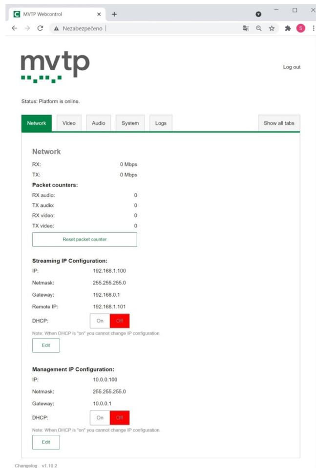
Fig. 2: Network tab of the built-in web interface
